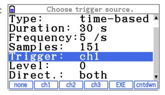
determine the state of the signal on the trigger channel to automatically start the measurement.
