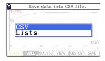
When saving via the SAVE option on the GRAPH screen the data of actual displayed graph are saved, quantities displayed along X-axis, Y-axis and 2nd Yaxis if exists.
