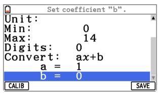
corresponding quantity value. Repeat for the second and, if present, the third calibration point. If the measured voltages of calibration points are too close you will be not able to enter a next calibration point.
