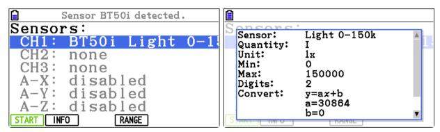
Left: The CMA Light sensor BT50i is automatically identified.
