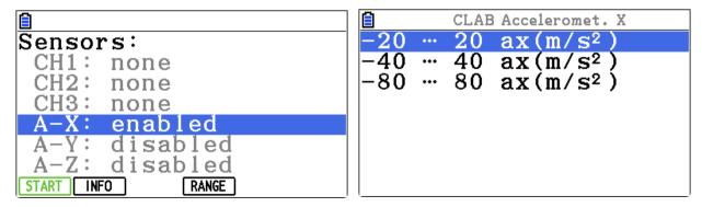
Left: The internal accelerometer in the direction  $\boldsymbol{X}$  is enabled.
