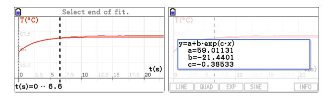
Left: The temperature measurement fitted with the exponential function. Right: The detailed information about the exponential function-fit displayed via the INFO option.
